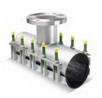
The SST is in fact a reinforced double band clamp with a flanged outlet. The standard working range is 20mm. The upper body is reinforced to accommodate the installation of valves and drilling equipment.
